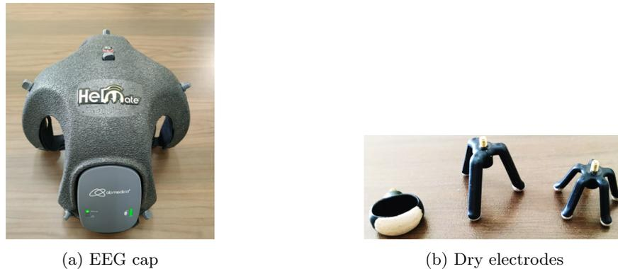
Fig. 2: EEG acquisition system.
